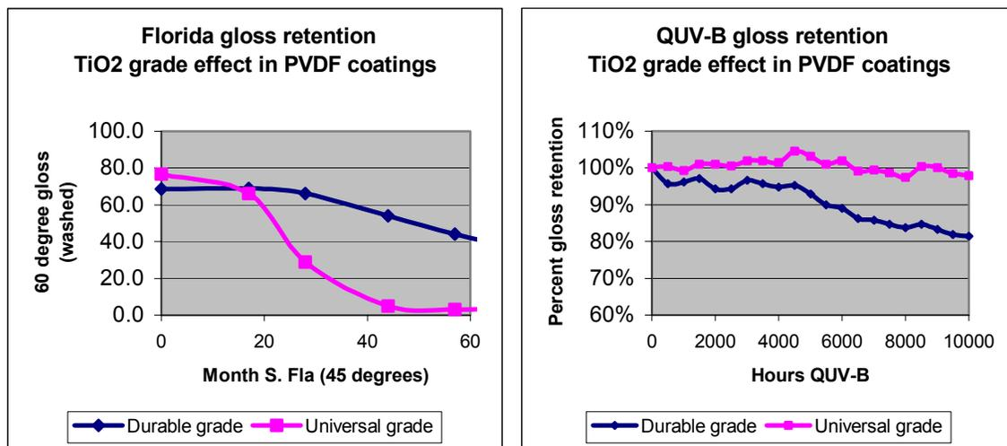
Figure 8. Comparison of Florida gloss retention and QUV-B retention, for two different grades of TiO<sub>2</sub>.
