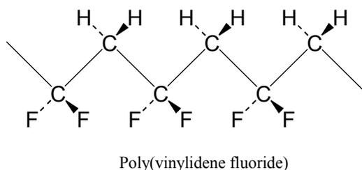
Figure 5. Structure of PVDF, or poly(vinylidene fluoride).
